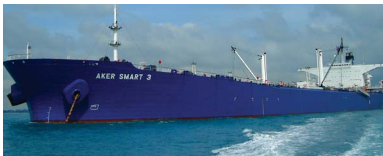
This 180,000-ton vessel serves as a stationary, floating storage tank.
